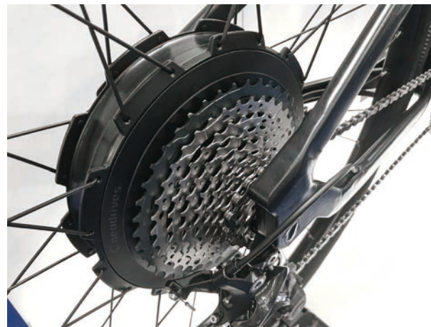
← Alber just released a improved version of its gearless rear hub drive system. Apart from some mechanical improvements, the display, remote control and software features have also been updated. The silent drive system is popular for touring bikes where motor noise is usually not well accepted by customers. (Source: Hannes Neupert)
