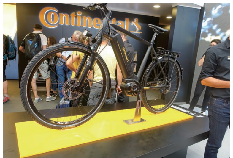
▲ Continental displayed its 48V drive system featuring stepless automatic transmission.
