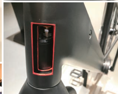
↑ ↑ ← ZF debuted their ultra compact and lightweight center drive system in a show case model made together with Canyon bicycle at IAA Frankfurt in September 2017. The showcase bike has had das well hidden in the frame tubes ABS actuators for the front and rear brake. (Source: ZF)
