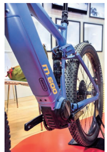
▲► Bafang's newest M500 & M600 drive system offer lighter weight and greater torque. They are specifically designed for eMTBs and Speed pedelecs. Taking power of 250W as an example, the motor now generates 95 newton-meters of torque, which is up from the 80 newton-meters of the past model. The motor's weight has been reduced from 3.9kg to only 3kg. Bafang has also added a new 500W motor generating 120 newton-meters, and provides built-in batteries.
