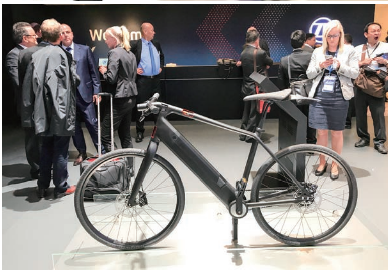
↑ ↑ ← ZF debuted their ultra compact and lightweight center drive system in a show case model made together with Canyon bicycle at IAA Frankfurt in September 2017. The showcase bike has had das well hidden in the frame tubes ABS actuators for the front and rear brake. (Source: ZF)
