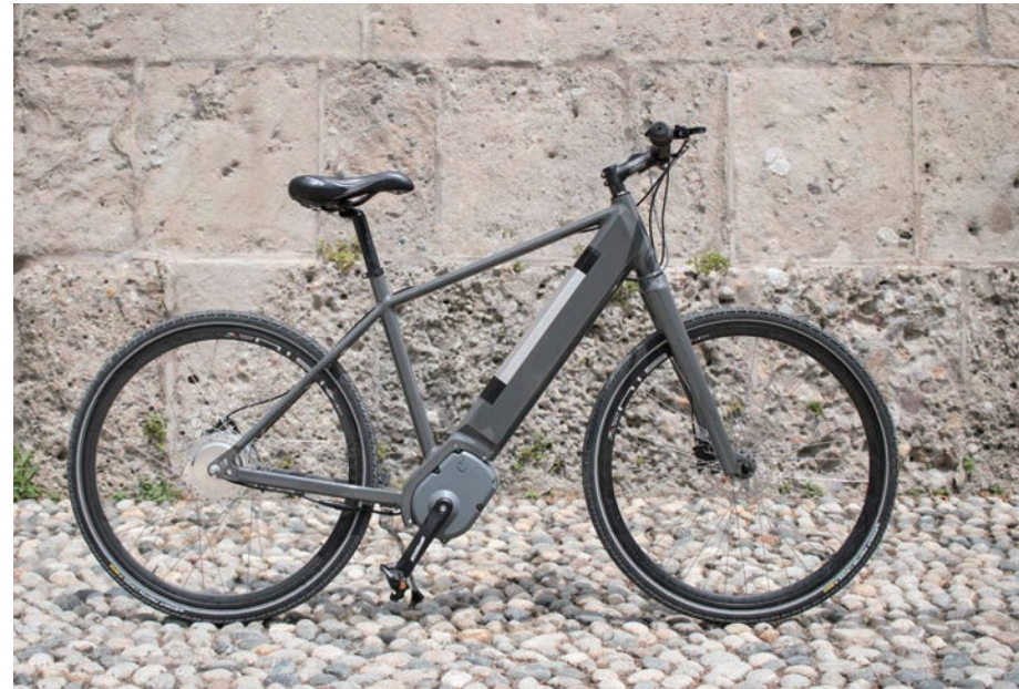
↑ The serial drive system maker Bike2 from Denmark claims to be ready for the market now after showing its system at several events. All of the big players in the bicycle industry still seem to ignore the fact that the serial hybrid drive train which works completely without a mechanical power transmission between the pedal and the wheel - has plenty of unique features that could make it THE drive system for next the generation of pedelecs. Several automotive players are working intensively on similar systems which will surface sometime soon. The biggest worry is the suggested low total efficiency - but in fact when considering that human efficiency can be improved quite substantially, the efficiency can be even higher than conventional mechanical drive trains. However, this seems counter-intuitive to most people at first. (Source: Bike2)
