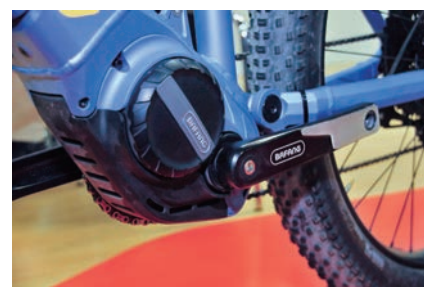
▲► Bafang's newest M500 & M600 drive system offer lighter weight and greater torque. They are specifically designed for eMTBs and Speed pedelecs. Taking power of 250W as an example, the motor now generates 95 newton-meters of torque, which is up from the 80 newton-meters of the past model. The motor's weight has been reduced from 3.9kg to only 3kg. Bafang has also added a new 500W motor generating 120 newton-meters, and provides built-in batteries.
