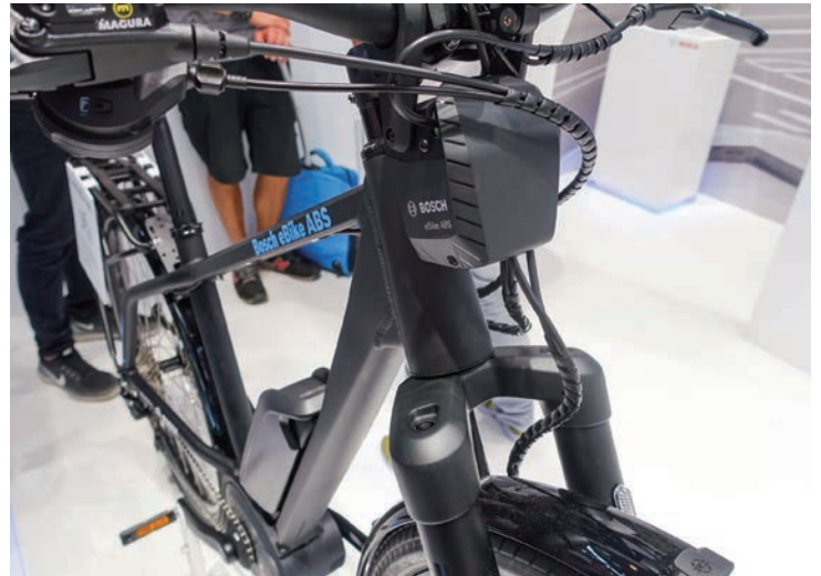
▲ Bosch have developed an ABS system designed for city, touring and trekking e-bikes.
