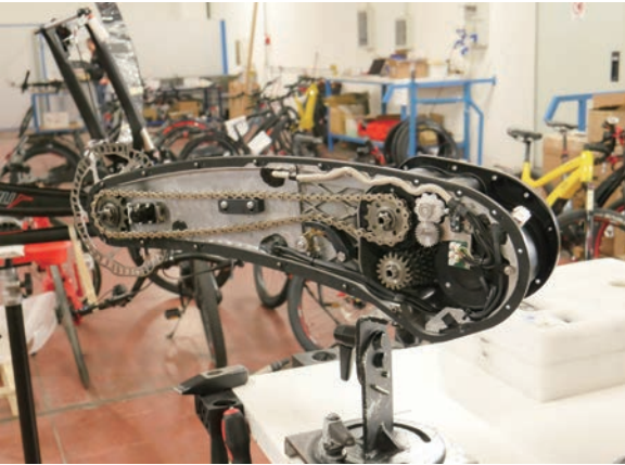
↑ The Neox drive system, which until now was only available in the Neox pedelec range offered by the north Italian maker, has several unique features like the integrated 8 speed gear system, a mechanical locking of the chain and an electronic disconnection of the bottom bracket as anti theft measures. Another great feature is the frame mounted disk brake which stays on the frame when the rear wheel is removed. Neox is welcoming inquiries from vehicle makers for their drive unit technology to be applied to other vehicles. (Source: Hannes Neupert)
